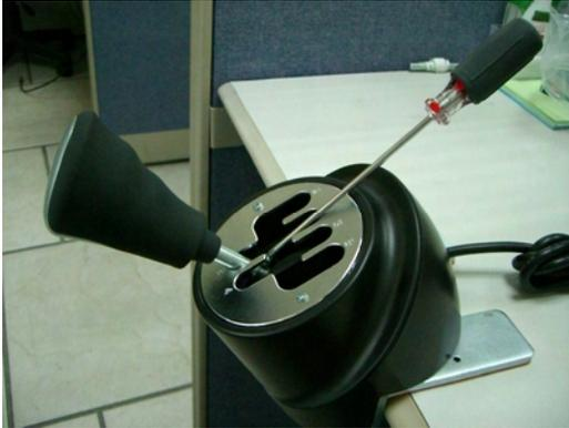
1. The first few steps for changing the gear plate are the same as removing the shifter knob. Refer to Steps 1 to 4 on page seven to remove the shift post.
